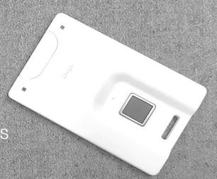
Zwipe Access is a versatile fingerprint-activated contactless credential working seamlessly with existing 125kHz or 13.56MHz infrastructure, without upgrading or replacing any readers or backend systems. Only after activation by a fingerprint scan will the card allow communication with a reader. Zwipe combines the security of biometric authentication with the speed and convenience of contactless credentials.
